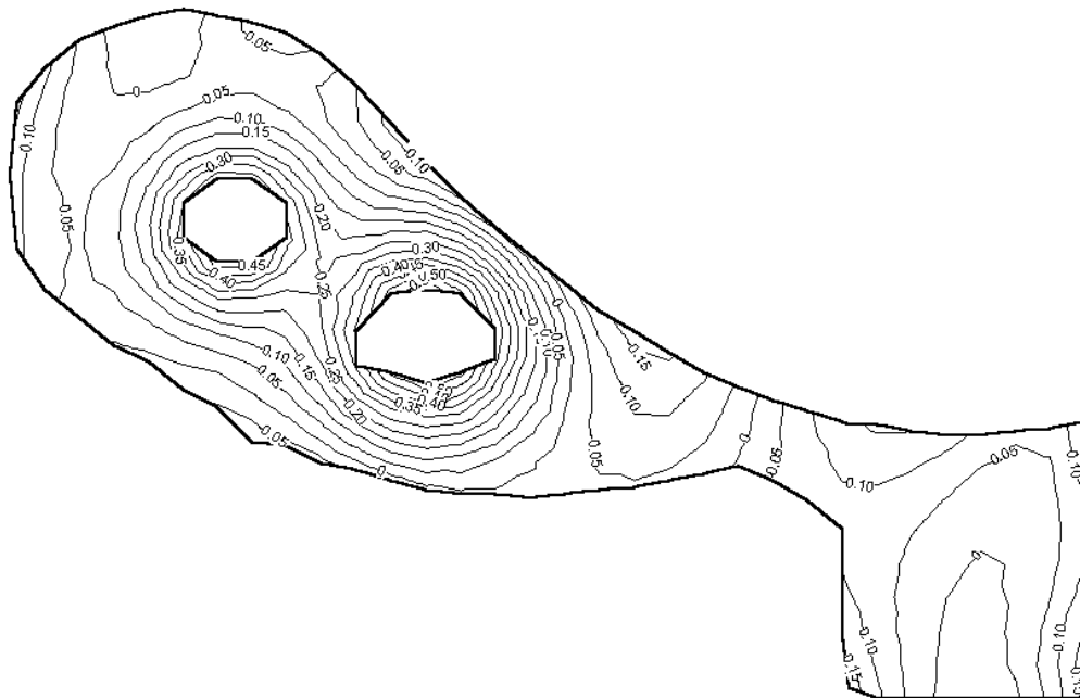
Figure 15. RVBEM Relative Errors (decimal) at X = 3.5 (local coordinate X^* = 19.67 ).
