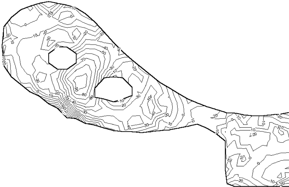
Figure 19. CVBEM Approximation Error at X = 6 (local coordinate X^* = 22.17 ).
