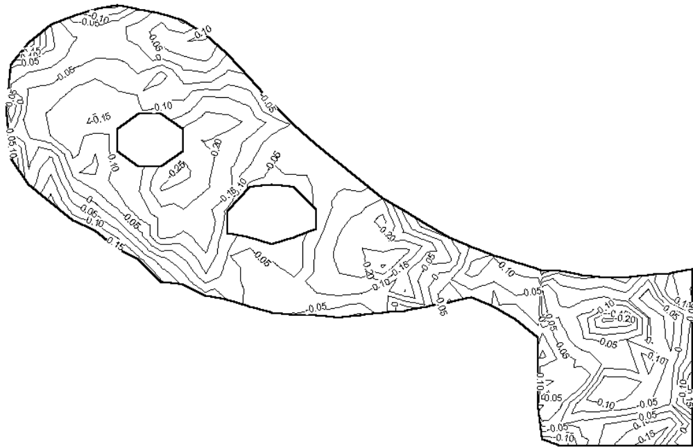
Figure 7. CVBEM Relative Errors (decimal) at X = 1 (local coordinate X^* = 17.17 ).
