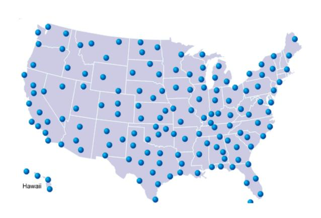
The Weather Surveillance Radar (WSR-88D) is the technical name for the 159 high resolution Sband Doppler weather Radar, which are part of the NEXRAD (Next **Generation Radar)** network
