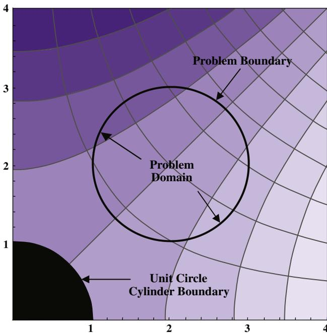
**Fig. 1.** FLOWNET of the Example Problem 1 Solution: The problem domain is the area enclosed in the problem boundary as shown. The problem domain is centered at (2,2). The unit circle cylinder boundary (shown as the boundary of the shaded quarter disk) is part of the boundary of the underlying ideal fluid flow around a 90 degree bend over a unit radius cylinder.
