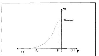
Figure 2. Conceptual Relationship Between Water Content (w) and Pore Pressure (P) for an Unsaturated Soil Media.
