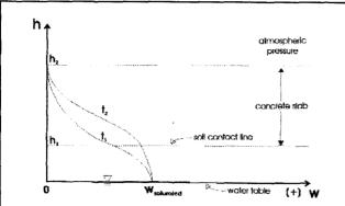
Figure 4. Conceptual Wetting Curves through a Concrete Slab for Various Times  $t_2 > t_1$ .
