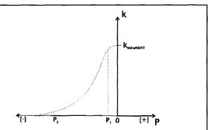
Figure 3. Conceptual Relationship of Hydraulic Conductivity (k) to Pore Pressure (P) for an Unsaturated Soil Media.
