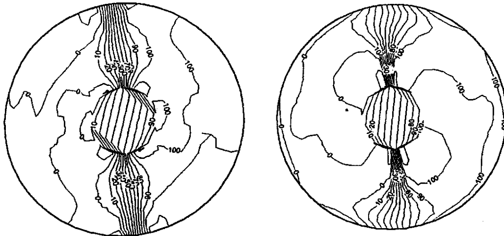
South Hemisphere Approximation of F(x,y,z) = 100 on East Hemisphere F(x,y,z) = 0 on West Hemisphere With Rotations I, II, III and IV
