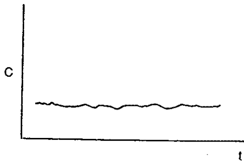
(b) Pollutograph with constant concentration
