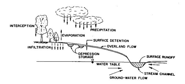
Figure 1. Watershed Runoff Cycle.
