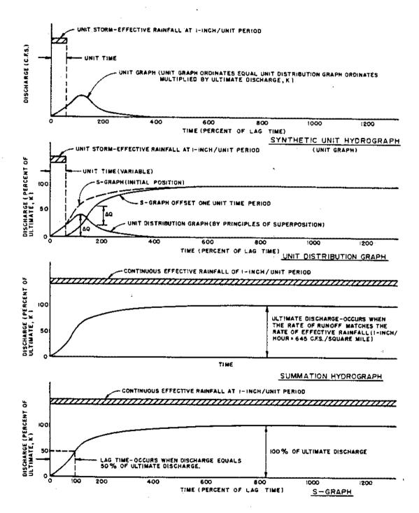
Figure 4. Definitions used in the Unit Hydrograph Concept
