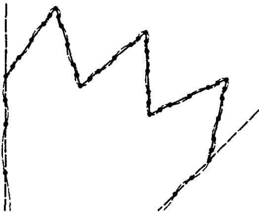
Fig. 8. Approximative Boundary (Dashed Line) After Four Attempts Using CVBEM. (Departures between \Gamma and \bar{\Gamma} are Magnified Tenfold)
