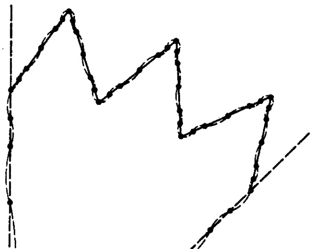
Figure 8. Approximative boundary (dashed line) after four attempts using CVBEM (departures between \Gamma and \hat{\Gamma} are magnified ten-fold)
